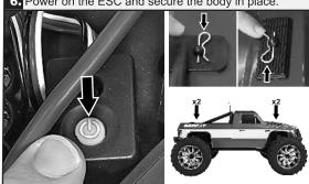
NOTE: You can also operate the ON/OFF switch by reaching under the body behind the front right tire.
