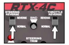
While driving away from you, if the vehicle steers to the left while you steer the controller to the right, reverse channel 1 by flipping the switch labeled "STEERING REVERSE". The switch labeled "THROTTLE REVERSE" is for reversing throttle orientation.
