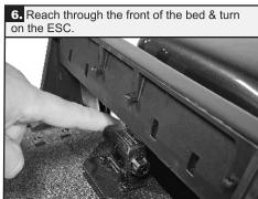
The ON/OFF switch is fastened to the front of the bed, behind the cab.
