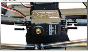
**8.** Using the Y-adapter included in the dual servo kit, connect both servos and put them into your preferred channel on the receiver. When using the included Redcat RTX-4C radio, put the Y-adapter into channel 3.
