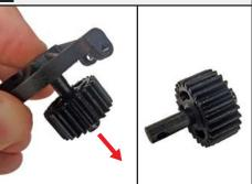
8. Pull the gear off of the lower idler shaft.
