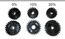
**10.** Put the new lower gear on lower idler shaft. (Will be either 24T, 25T, or 26T depending on your choice) (see step 9)
