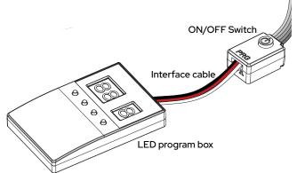
Using the LED program box to set ESC parameters.
