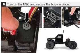
NOTE: You can also operate the ON/OFF button by reaching under the front right fender.
