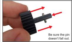
**11.** Put the lower idler shaft into the rear case.
