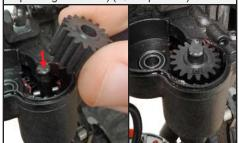
**13.** Realign the rear case and gently push it into place. (you may need to rotate the idler shaft slightly to line up the gears)
