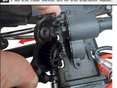
6. Angle the front of the chassis down and pull the upper gear out of transfer case. (Angling the chassis helps to keep the gear pin from falling out of the idler shaft.)
