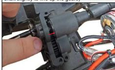
**14.** Reinstall the two screws. The longer screw goes into the driver's side of the case and the shorter screw goes into the passenger's side.
